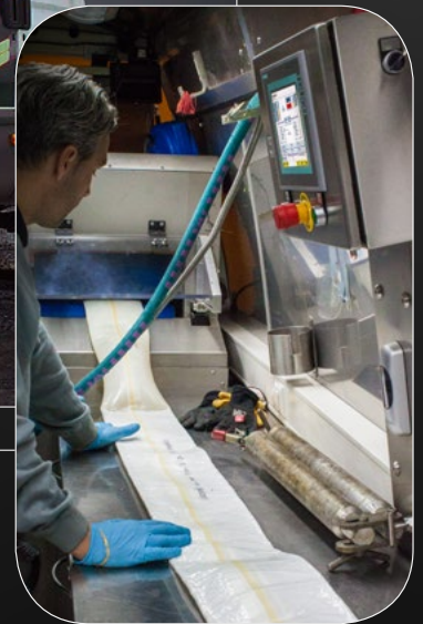
Mixing Unit: RS CCM ® incl. calibration roller
